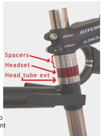
(Illustration at right) Shows a 10mm simulated head tube extension, a red 15mm spacer to simulate a threadless upper headset plus 20mm of headset spacers, over which you mount the stem and bars.
