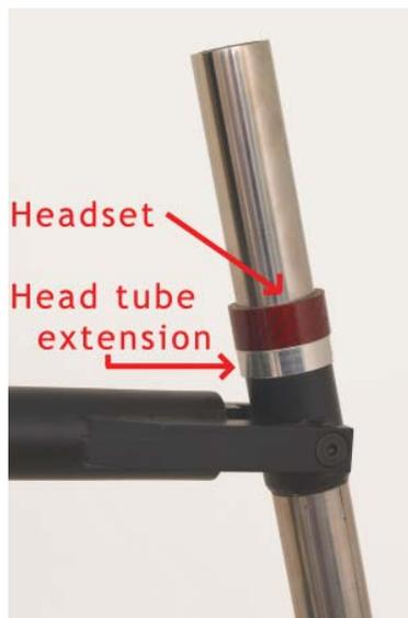
(Illustration at center) Simulates a 10mm head tube extension with a 15mm simulated threadless upper headset.
