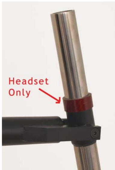
(Illustration at left) Shows a red 15mm spacer to simulate a threadless upper headset. Integrated headsets use a smaller stack (typically 6mm).
