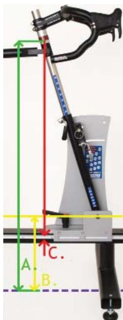
**Slowtwitch.com Stack and Reach Measurements (left):** The bottom of the red headset spacer indicates the top of the head tube. This is the target measurement position for Stack and Reach Measurements:
