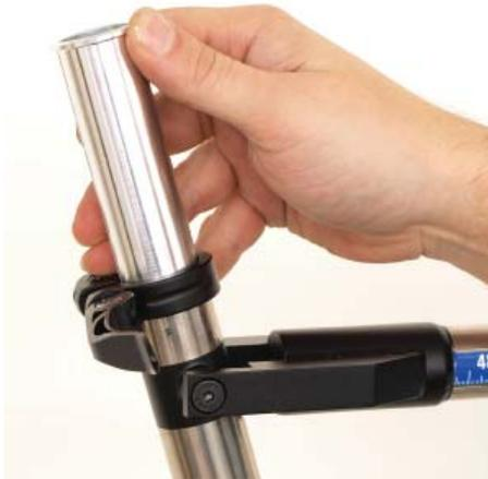
Insert the seat tube insert (which insures a proper fit-up with 27.2mm seat posts). Then slip the quick-release clamp over the assembly. You are now ready to install a seatpost.
